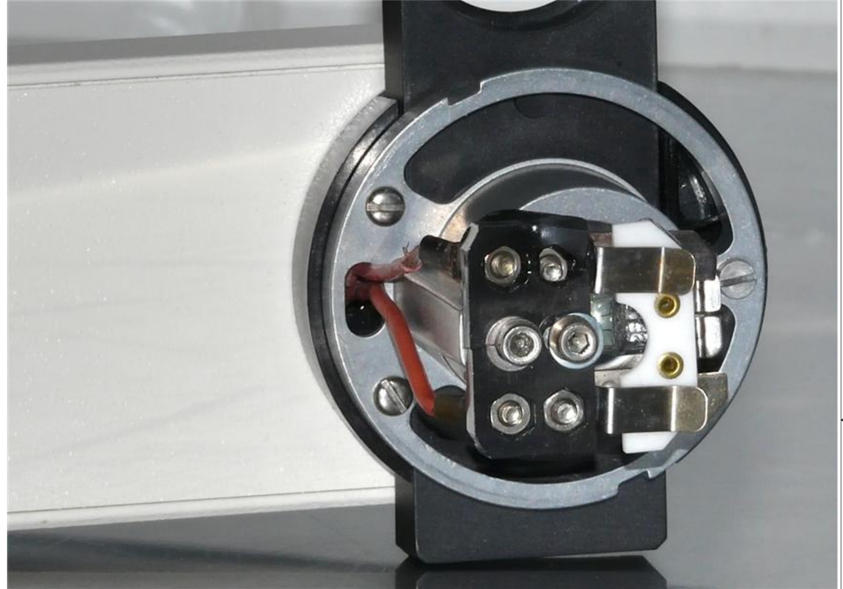
(2) Note the three screws holding the lamp/collector lens assembly in place.
